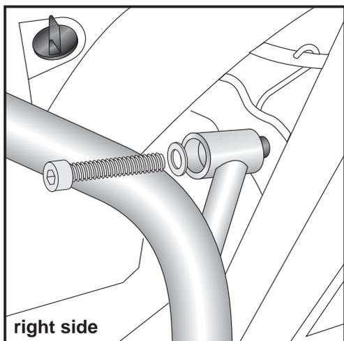
**2** Fastening of the engine guard middle left + right:
