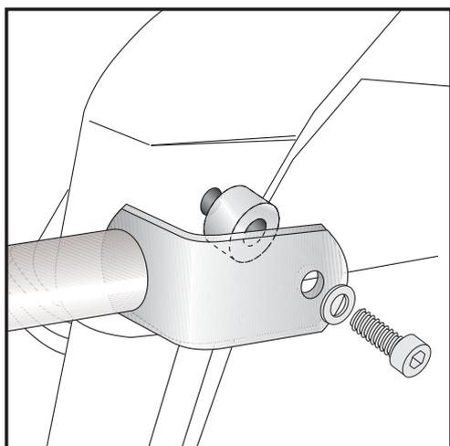
**3** Fastening of the engine guard top left + right:
