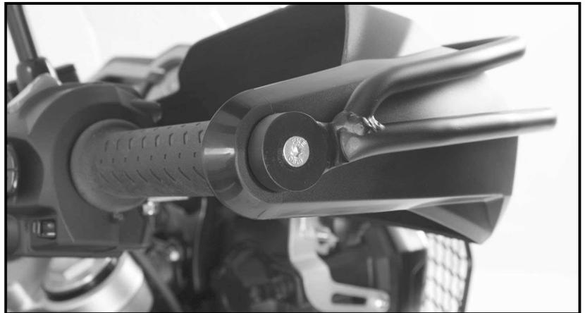
Fastening of the handle protection bar left and right top:
