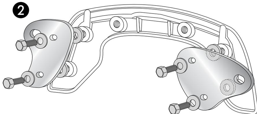
**2** Fix the C-Bow with mounted adapters at the chrome bar of the bike.
