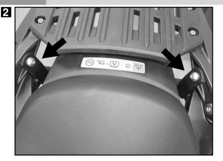
Fastening of the C-Bows left and right: at the adapters. Align the adapter so that the holes matches the threads in the wings.
