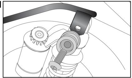
Fastening of the C-Bow on the right: use hexagon bolts M6x18 with washers Ø6,4.
