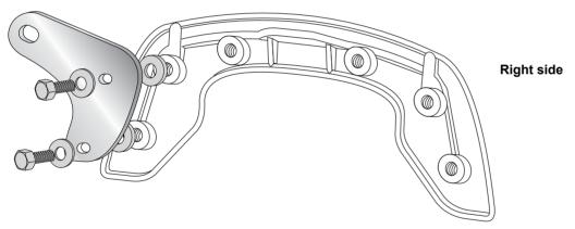
Fix the C-Bow to the chromed bar. Use filister head screws M8 x 75 with washer ø8,4. Sandwich spacer ø18 x ø9 x 35 mm.
